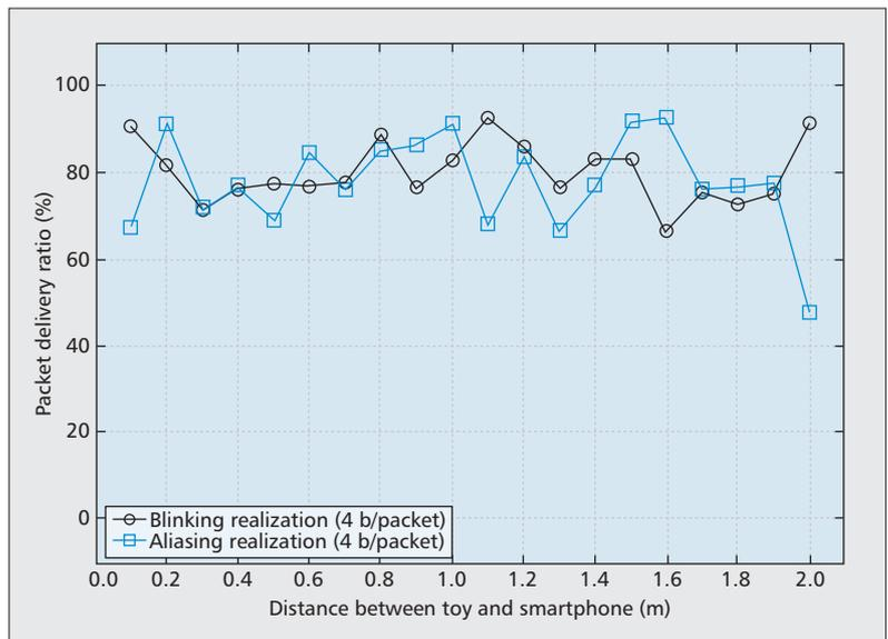
**Figure 5.** LED-to-smartphone communication mode: PDR over distance for an LED communicating to a camera; throughput: up to 1 b/s. Results are shown for distances of up to 1.5 m. The measurements result in the same packet loss ratio for both methods. However, the throughput is lower for the aliasing method because of the lower data rate (0.5 b/s and 1 b/s, respectively).
