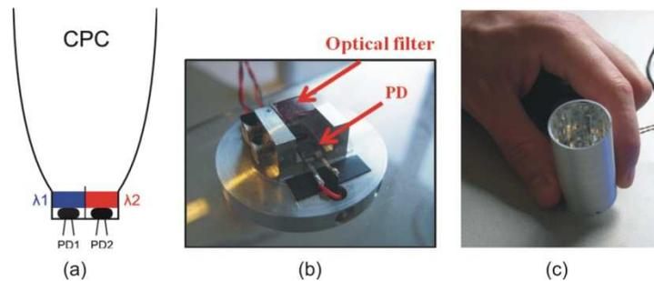
Fig. 2. Light collector. (a) Scheme of the collector stage: sensors (PIN photodiodes), wavelength filters  $\lambda_1$  and  $\lambda_2$  and CPC on top of the sensors. (b) Photodiode support. (c) Collector stage as implemented in the experiments.
